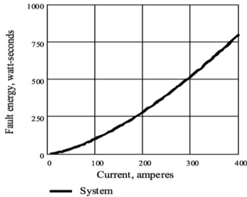
Fig. 7a. Energy due to “System Current – for Various Magnitudes of Current
