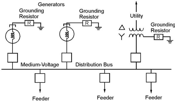
Fig. 1. Medium-Voltage Industrial Distribution System with Multiple Sources
