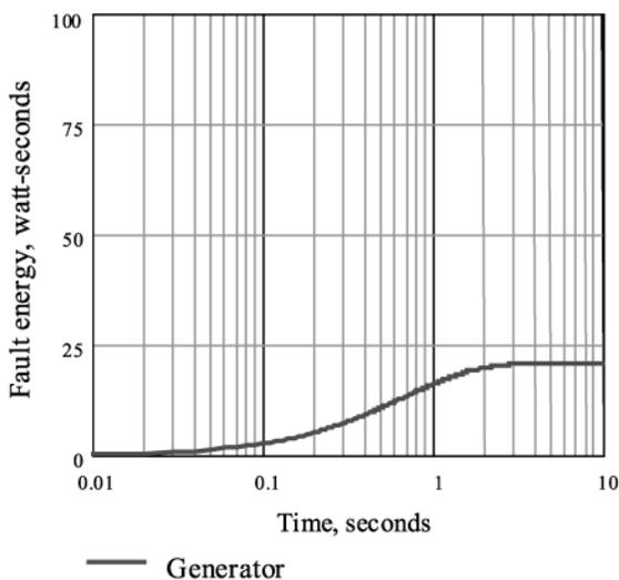
Fig. 9. Fault Energy Versus Time with 10A Grounding
