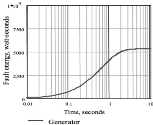
Fig. 8b. Arc Energy due to 400 A “Generator Current” Over Time
