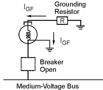
Fig. 2. Generator Internal Ground Fault – Current Flow after Opening Generator Breaker
