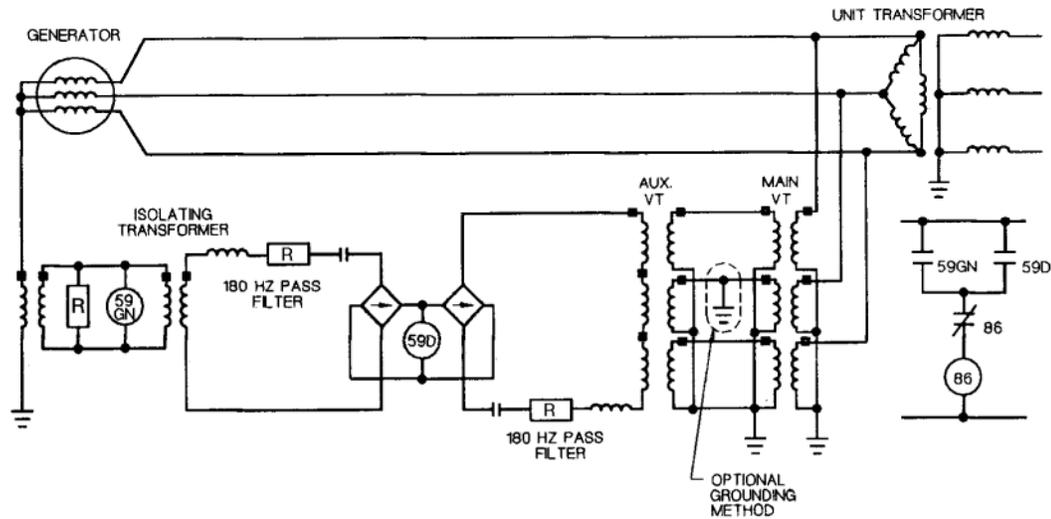
59GN Overvoltage Relay Tuned to the Fundamental (60 Hz) Frequency
