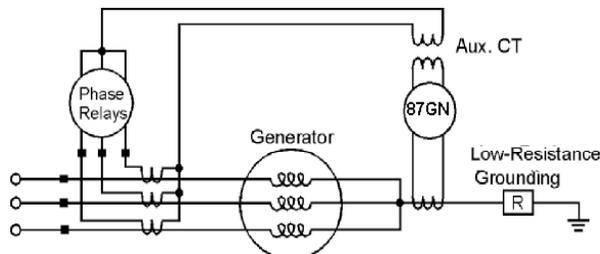
Fig. 20. Generator Ground Differential Protection
