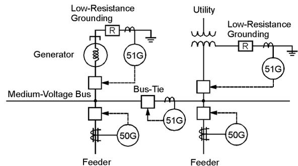
Fig. 21. Generator Ground Time Overcurrent Protection
