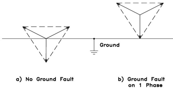
Fig. 13. Voltages During Ground Fault on Ungrounded System
