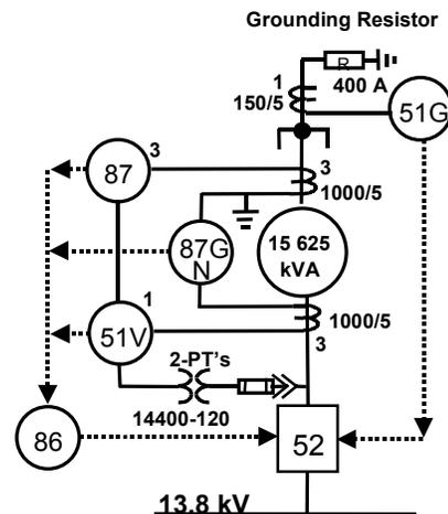
Fig. 3. Simplified Single-line Diagram of Example System
