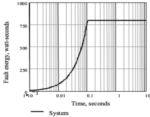
Fig. 7b. Arc Energy due to 400 A “System Current” Over Time
