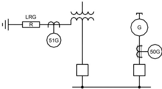
Fig. 15. Generator Ungrounded and System Low-Resistance Grounded
