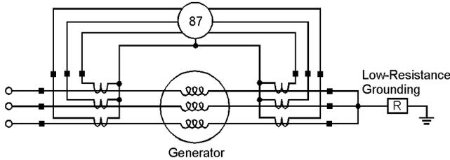
Fig. 19. Generator Percentage Phase Differential Protection
