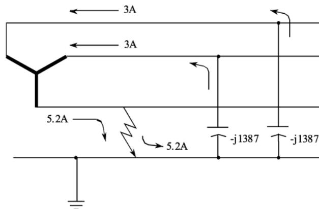
Fig. 12. Ground Faults on Ungrounded Systems
