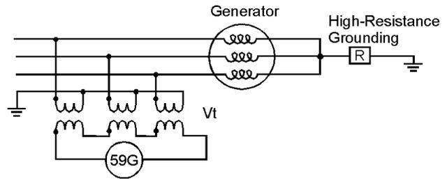
Fig. 23. Wye-Broken-Delta Vt, Ground Overcurrent Protection
