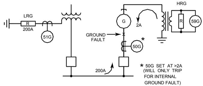
Fig. 16. Generator High-Resistance Grounded and System Low-Resistance Grounded
