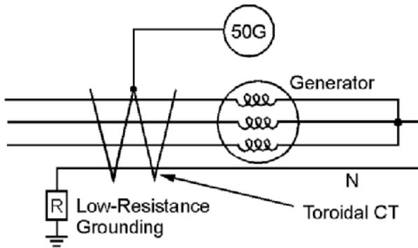
Fig. 22. Instantaneous Ground Overcurrent (Self-Balancing Differential Ground Current) Protection
