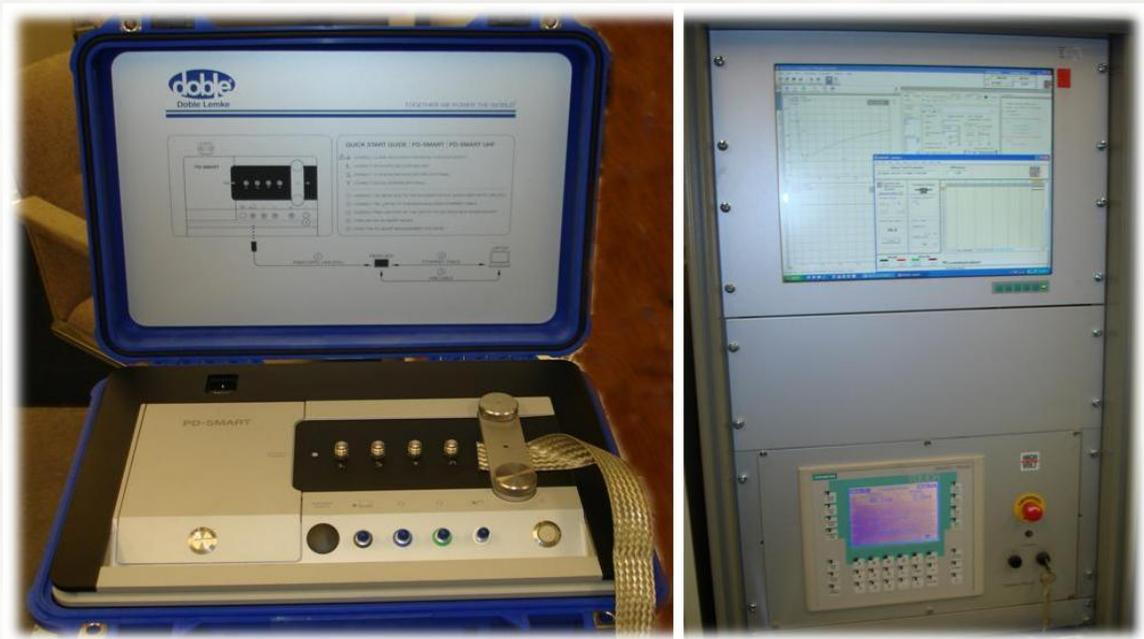
**Doble partial discharge (PD) test equipment**
