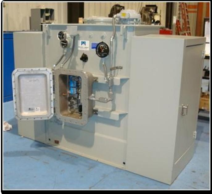
This photo provides a view of a transformer which has been constructed for installation in a hazardous environment. The gauge wiring has been enclosed in solid or flexible conduit in route to the explosion proof terminal box.
