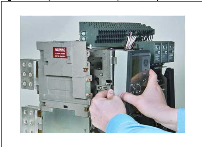
Figure 11. Trip Unit Removal Sequence, Step B
